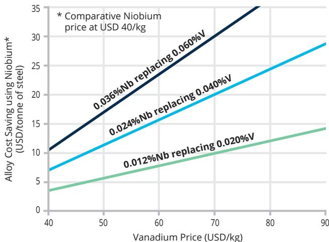
Note that the figure serves as a guide to the amount of alloy replaceable by niobium and that the relationship is not equal, i.e. one for one. The exact amount will depend upon the product type, final property requirements and steel-mill processing conditions. Nonetheless, typically 30% to 50% less alloy by wt.% is necessary to achieve the same strengths using only niobium.
